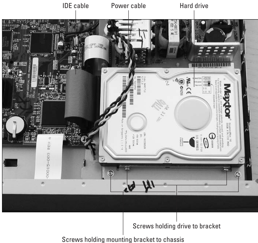
Figure 12-3: Examine TiVo to locate its hard drive, drive bay, IDE cable, power cable, and anything else listed in your kit's instructions.
